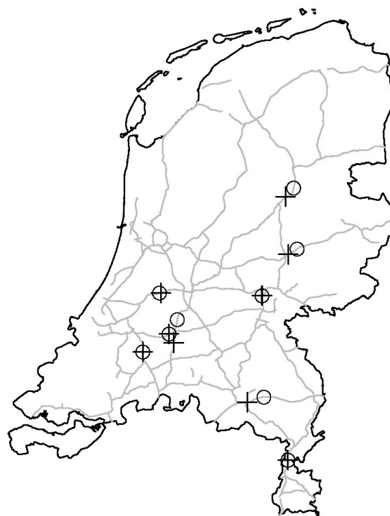
Fig. 1. Road sensor network on Dutch highways consisting of nine different systems with 18 measurement stations. Crosses and circles indicate the two stations of the nine WiM systems.
